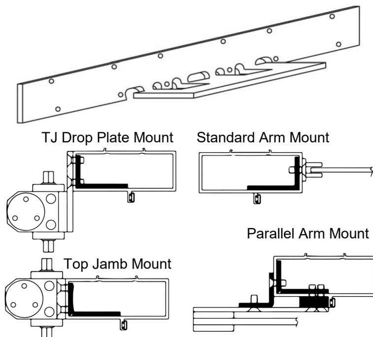
One plate can accommodate up to 4 different mounting positions
